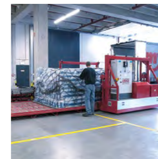
FlexLoader arvato Disribution Centre, Düren (Freight handling)
