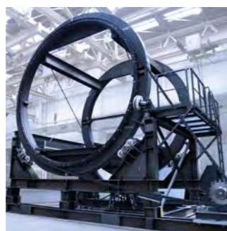
360° tilt mechanism for organic waste containers
